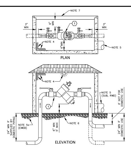
APPROVED DOUBLE CHECK VALVE ASSEMBLY INCLUDING FACTORY SUPPLIED SHUT-OFF VALVES: AS LISTED ON THE CURRENTLY APPROVED BACKFLOW PREVENTION ASSEMBLIES LIST SPECIFIED BY OREGON HEALTH AUTHORITY.
