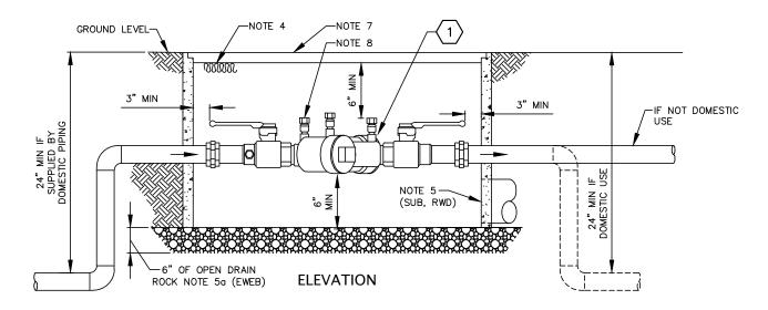
1 APPROVED DOUBLE CHECK VALVE ASSEMBLY INCLUDING FACTORY SUPPLIED SHUT-OFF VALVES: AS LISTED ON THE CURRENTLY APPROVED BACKFLOW PREVENTION ASSEMBLIES LIST SPECIFIED BY OREGON HEALTH AUTHORITY.
