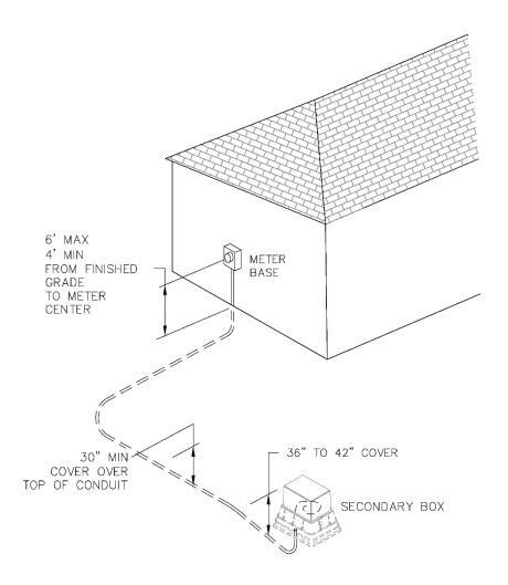
SINGLE PHASE SERVICE CONDUCTOR & CONDUIT SIZES
