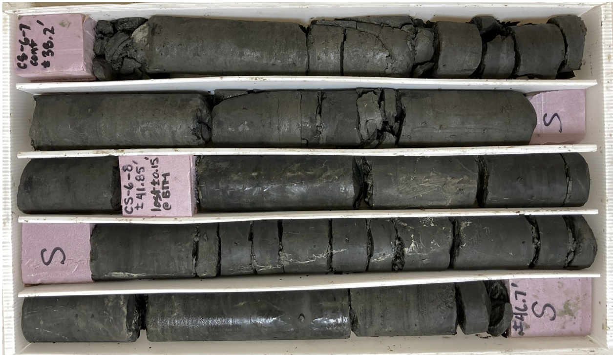
Photo 22B. BH-6 from 38.2 to 46.7 ft - Box 4 of 5
