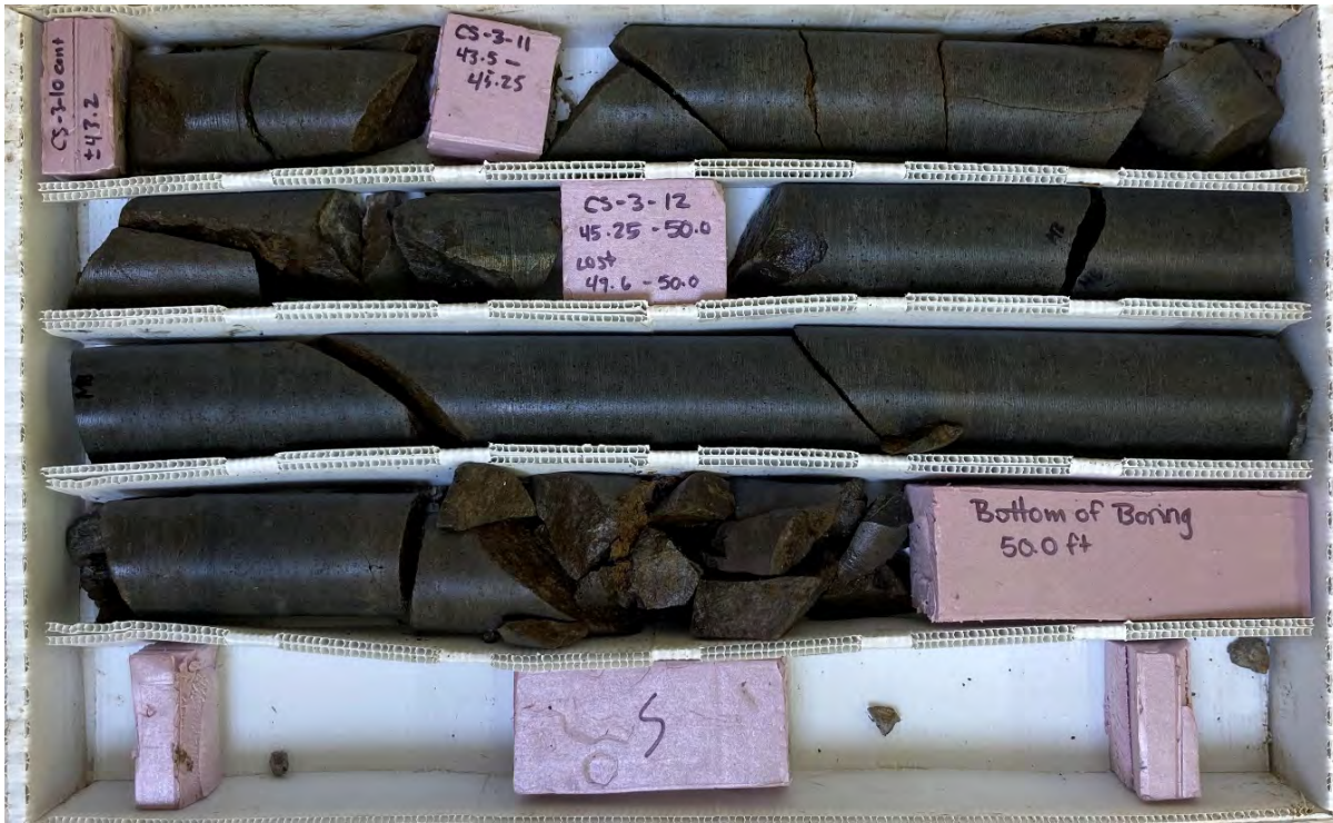
Photo 15B. BH-3 from 43.5 to 50.0 ft - Box 5 of 5
