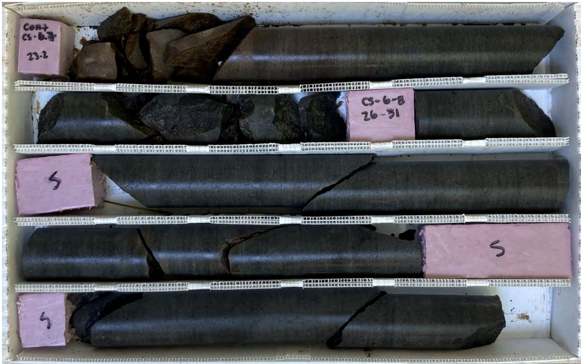
Photo 25B. BH-6 from 23.2 to 31.0 ft - Box 3 of 5
