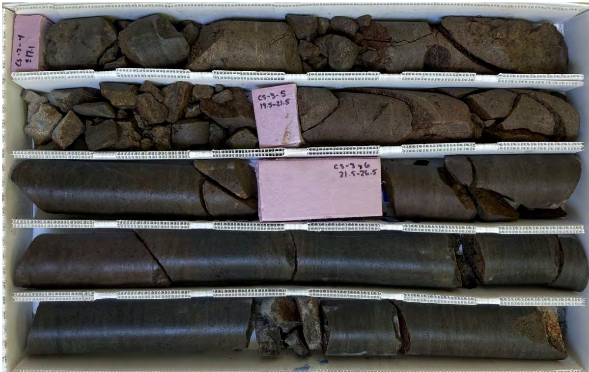
Photo 12B. BH-3 from 17.1 to 25.4 ft - Box 2 of 5
