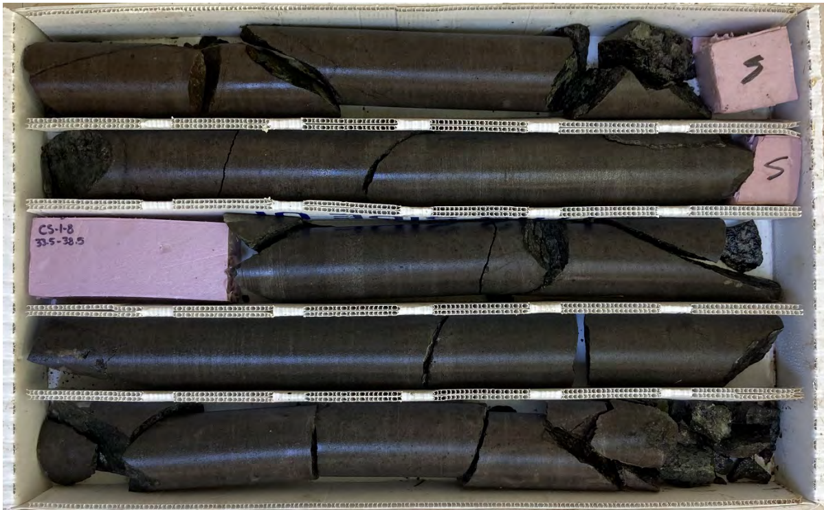
Photo 3B. BH-1 from 30.9 to 38.5 ft - Box 3 of 5
