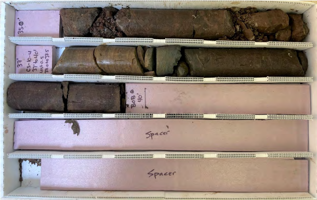
Photo 39B. BH-10 from 35.0 to 40.0 ft - Box 2 of 2
