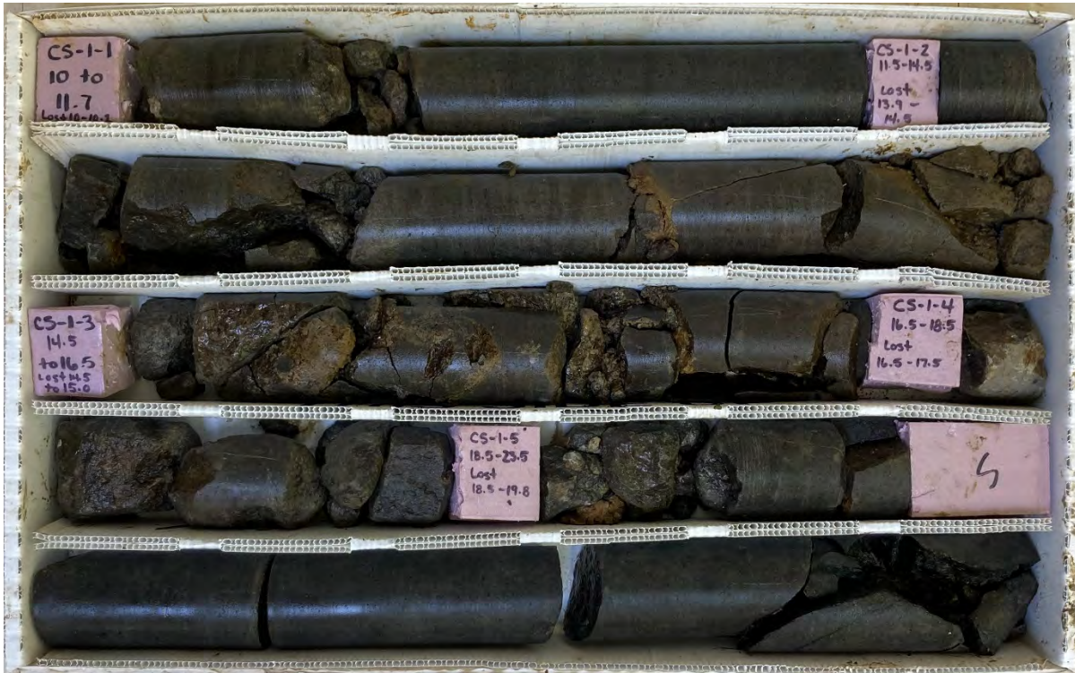
Photo 1B. BH-1 from 10.0 to 23.3 ft - Box 1 of 5
