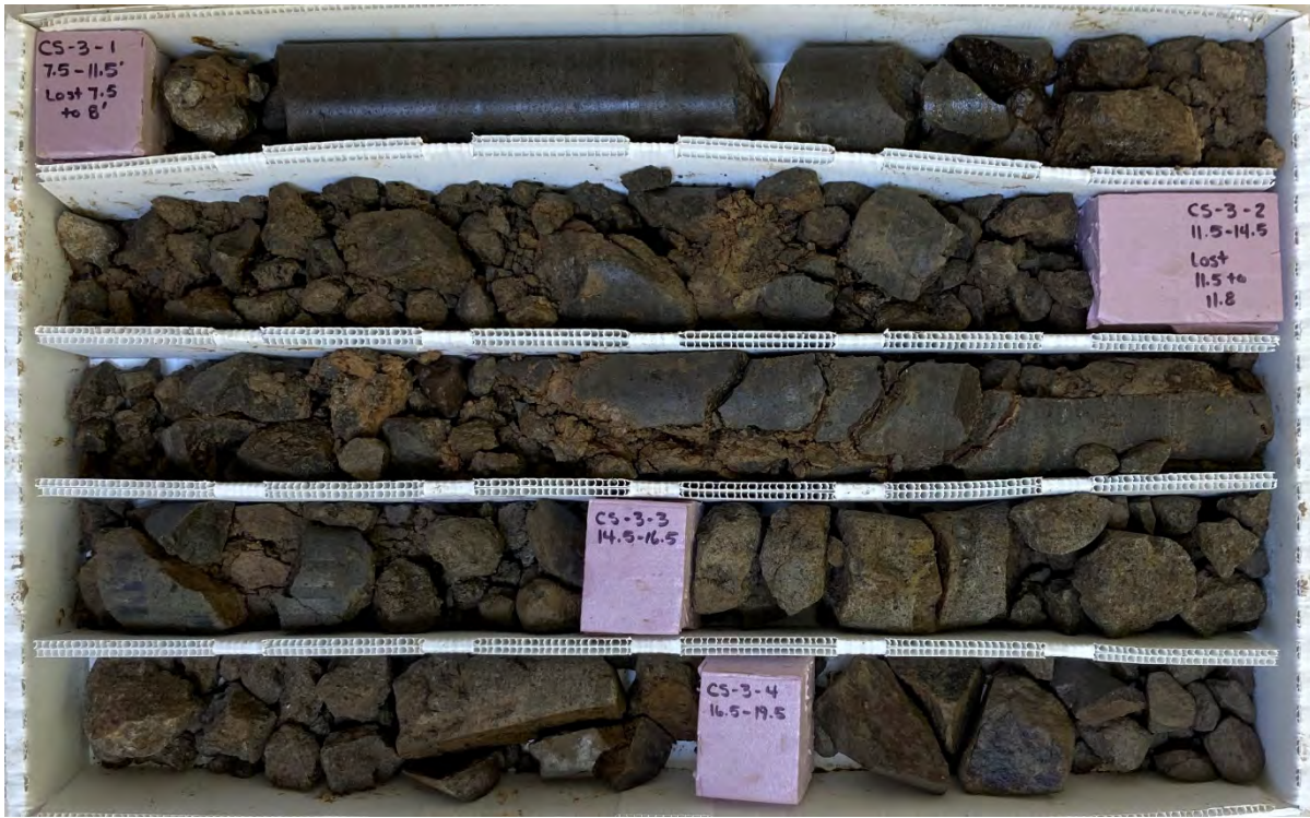
Photo 11B. BH-3 from 7.5 to 17.1 ft - Box 1 of 5
