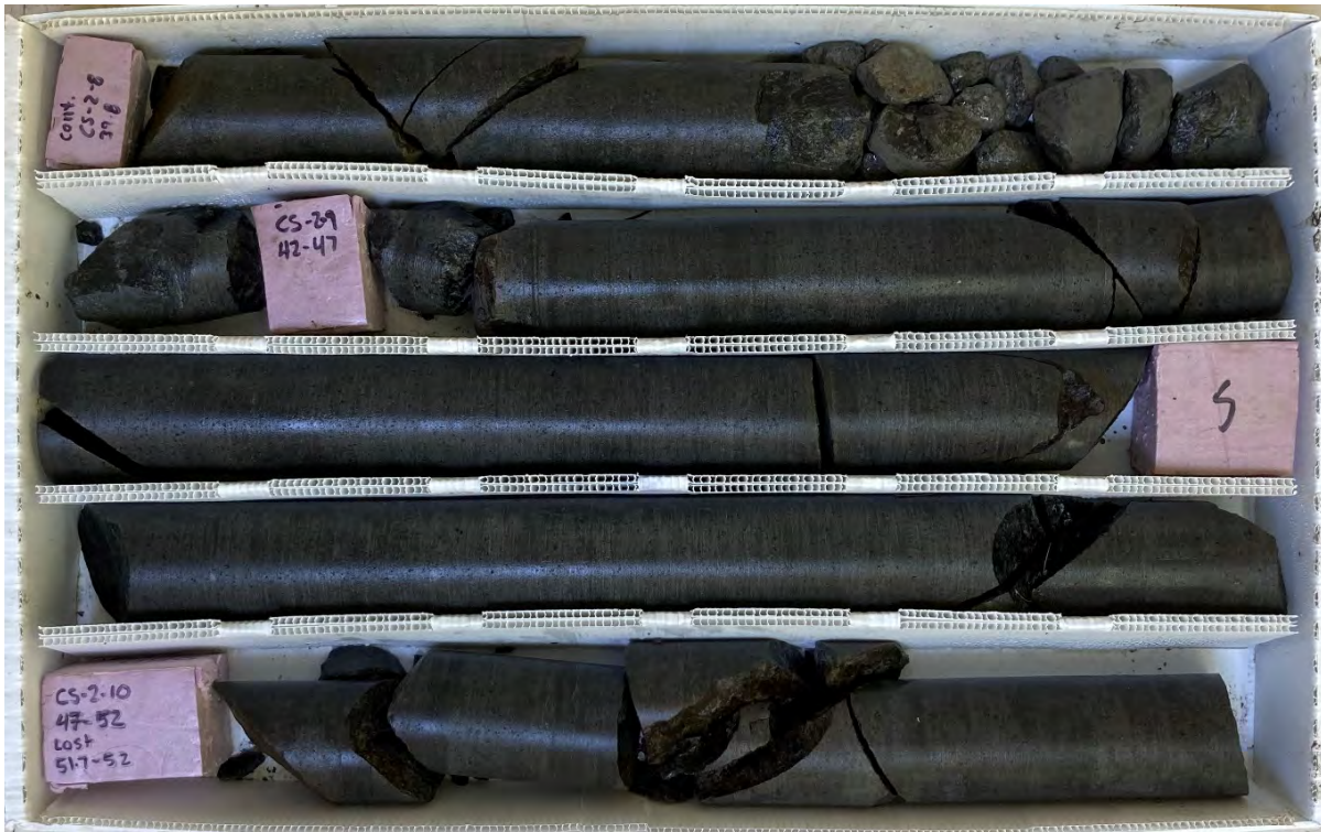
Photo 9B. BH-2 from 39.8 to 48.8 ft - Box 4 of 5
