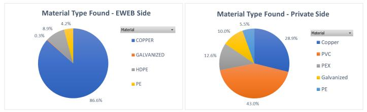
GALVANIZED = steel or iron pipes dipped in a zinc coating; HDPE = High Density Polyethylene; PE = Polyethylene; PVC = Polyvinylchloried; PEX = cross-linked polyethylene
